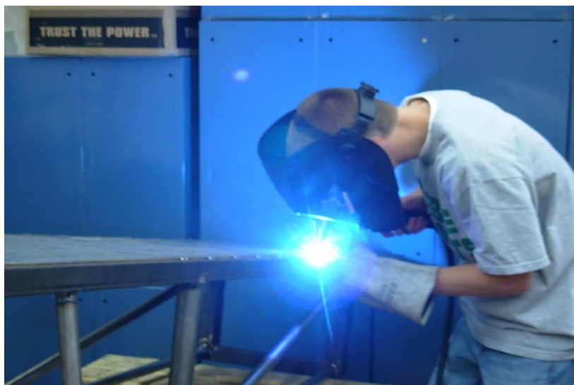
Jim Rettler welding the floor onto the chassis
